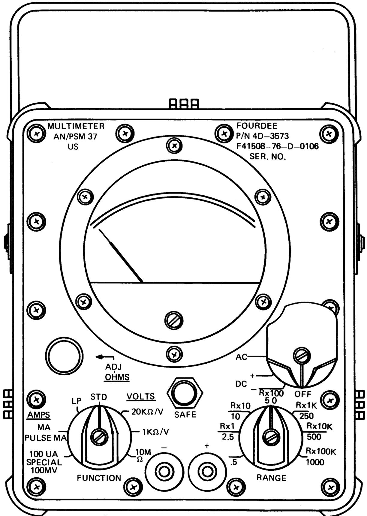
Figure 4-11. AN/PSM-37 multimeter controls
